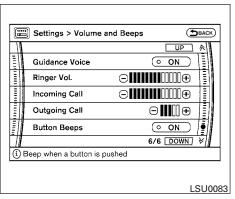
To access the settings, press the SETTING button, then highlight "Volume and Beeps" using the NISSAN controller and press the ENTER button.
